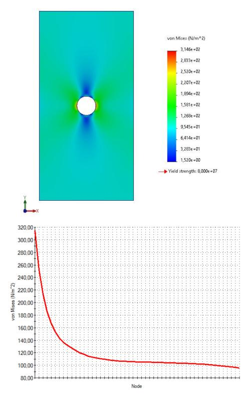
As can be seen on the graph, the stress is the highest closest to the ellipse, and quickly falls off the closer it reaches the edge of the plate, furthest away from the ellipse.
