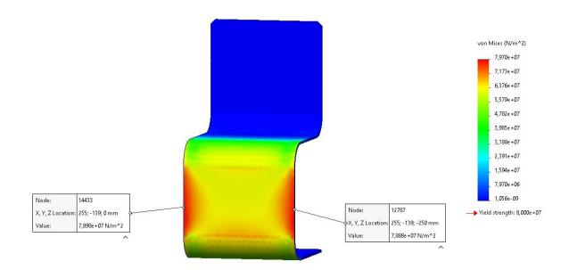
It is obvious where the largest load is when using the *Design Insight* tool. Meanwhile, the loading on the non-blue marked area is close to none. By reinforcing the area experiencing all of the load, the rest of the chair can remain with a thickness of 2.5mm.
