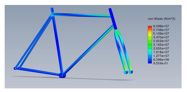
these changes, at the cost of adding 15 grams to the mass, make it so that the frame can withstand the load without reaching the yielding of 80 MPa, with the total mass being 1255g.
