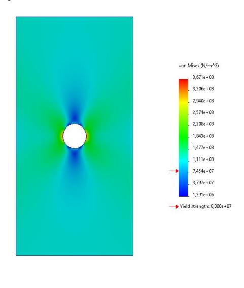
By instead applying  $\sigma_0$  with a value of 111 MPa the resulting maximum stress was 349.3 MPa, very close to the failure moment. That means that the approximated value 116.67 was over 5% than what was needed by simulation
