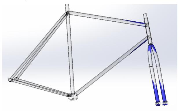
The highest stress concentration comes from sharp edges, these are dealt with by rounding the sharp edges with *fillets*. Fillets would come during production from welding the pipes together.
