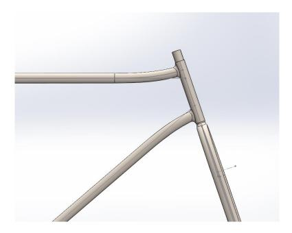
This ellipse shape of tubing was also applied to the tubes at the front, a similar 20mm height, 10mm wide shape with a 2mm wall thickness was found to be strong enough to withstand the load, while also bringing the mass down to 693 grams.
