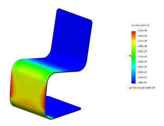
If a 100kg person sits on the chair, the largest von mises effective stress is 151 MPa. If the strength of the material is 80 MPa, the maximum safe force would be 550N, which translates to 56 kg. The failure would occur first at either side of the bottom half, shown in red.
