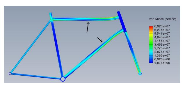
Also applied was a slight angle between the connection of the *main frame* and the front. The idea was to compensate for the load that can be seen on the top side of the upper tube, and the bottom side of the lower tube. This proved to be a positive change, and is very much doable in a manufacturing perspective, by simply bending the tubes.
