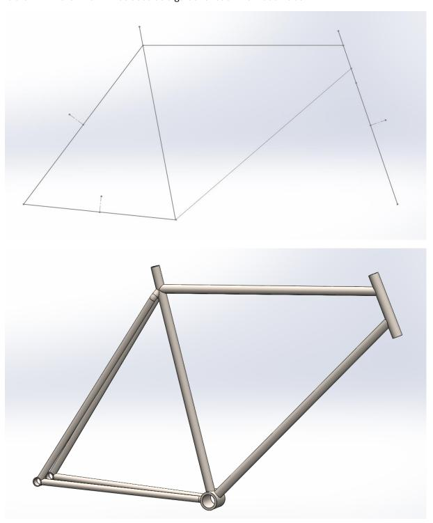
The main frame was created by using the sweep tool, creating pipes that are 20mm wide in diameter with 2mm thick walls. Exception to this is the supporting frames for the back wheel, which are 14mm wide in diameter (but still 2mm thick).
