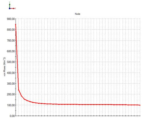
a = 10 mm and b = 0. The maximum simulated von Mises stress reached 2332 N/m², whereas the formula for the approximation contains a division by zero which means that the maximum stress would go towards infinity. Because of how meshing works, SolidWorks has to assume a certain size, even though you may limit that mesh size to say  $0.01 \text{mm}^2$  cubes, it can never be zero and therefore the max stress will not reach values close to infinity.
