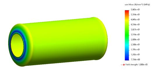
By probing the middle section of the pipe, an average of 45.04 MPa was measured. This value was very close to the theoretical solution. Where it does differ is at the maximum measured values, which in the simulation measured up to 58.36 MPa, much higher than the theoretical solution. These high stress points were found at the edges of the pipe and may lead to failure if not taken in to account while designing the pipe.
