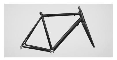
A bicycle frame is to be manufactured from Aluminum. The elastic modulus and Poisson's ratio of the material are E=70 GPa and  $\nu=0.3$ , the strength is  $\sigma_f=80$ MPa and the density is 2700kg/m³. The frame shall be able to bear a weight of m=150kg in the vertical direction when it is in use, and it can be assumed that this total weight is distributed as  $P_1=0.4m$ ,  $P_2=0.3m$ ,  $P_3=0.3m$ , as shown in the figure below.
