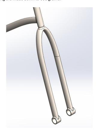
Here is a picture of the final designs simulation, with a maximum effective stress of 65.19 MPa. The final weight of the frame is 693 grams.
