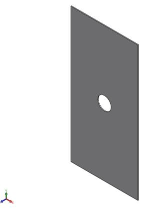
The simulation was set up as a 2D simplification, to achieve plane conditions and simulation on a 2D shape. A pressure of 100 N/m<sup>2</sup> was applied as  $\sigma_0$  on the bottom and the top side of the plate (y-direction)
