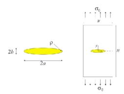
A plate of length H and width W is under tension in the y direction, and the remote tensile stress is  $\sigma_0$ . At the center (x = y = 0) of the plate, there exists a defect which takes the shape of an ellipse with halfaxes a and b. When a = b, the defect is a circular hole, and when  $b \to 0$ , it becomes a crack.
