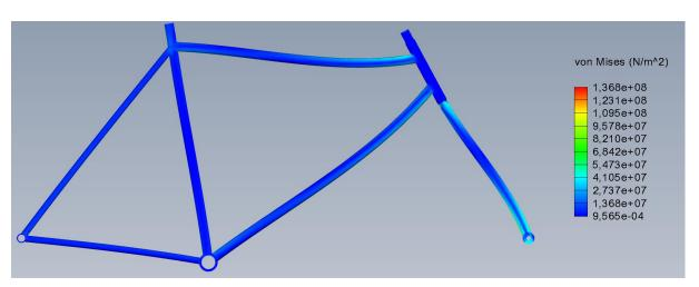
This will be used as a starting point, from which an attempt will be made to improve the design so that it can withstand the load, while minimizing mass. The current mass is 1240 g.
